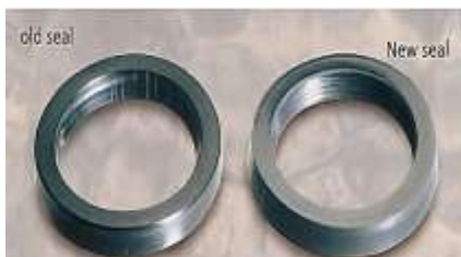
Figure 21 the Contamination Damage in Rod Seal
